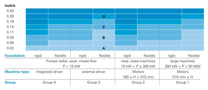
DIN ISO 10816: Mechanical vibrations – assessment of the vibrations of machine through measurements on no rotating parts. Vibration velocity (rms) 10 - 1000 Hz, n > 600 min<sup>-1</sup>, 2 - 1000 Hz, n > 120 min<sup>-1</sup> **A** = new machine condition **B** = unlimited long-term operation allowable **C** = short-term operation allowable **D** = Vibration causes damage
